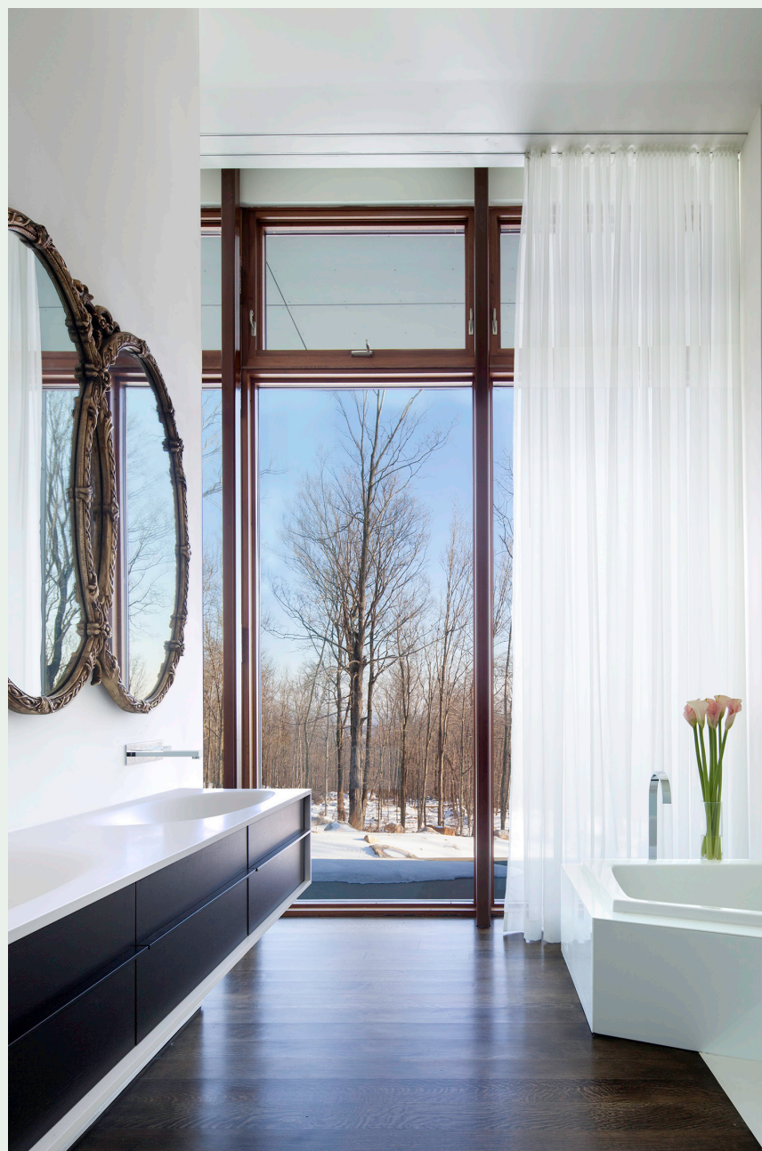
Efficient quadruple-paned windows were part of the building's overall sustainable material choices that helped lead to a LEED Silver certification.
